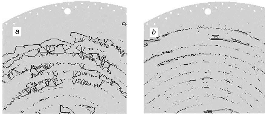
Fig. 7. A part of the antenna with distribution of the ultrahigh frequency current over the main slot transmitters.
