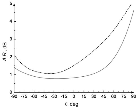
Fig. 4. Axial ratio of the antennas.
