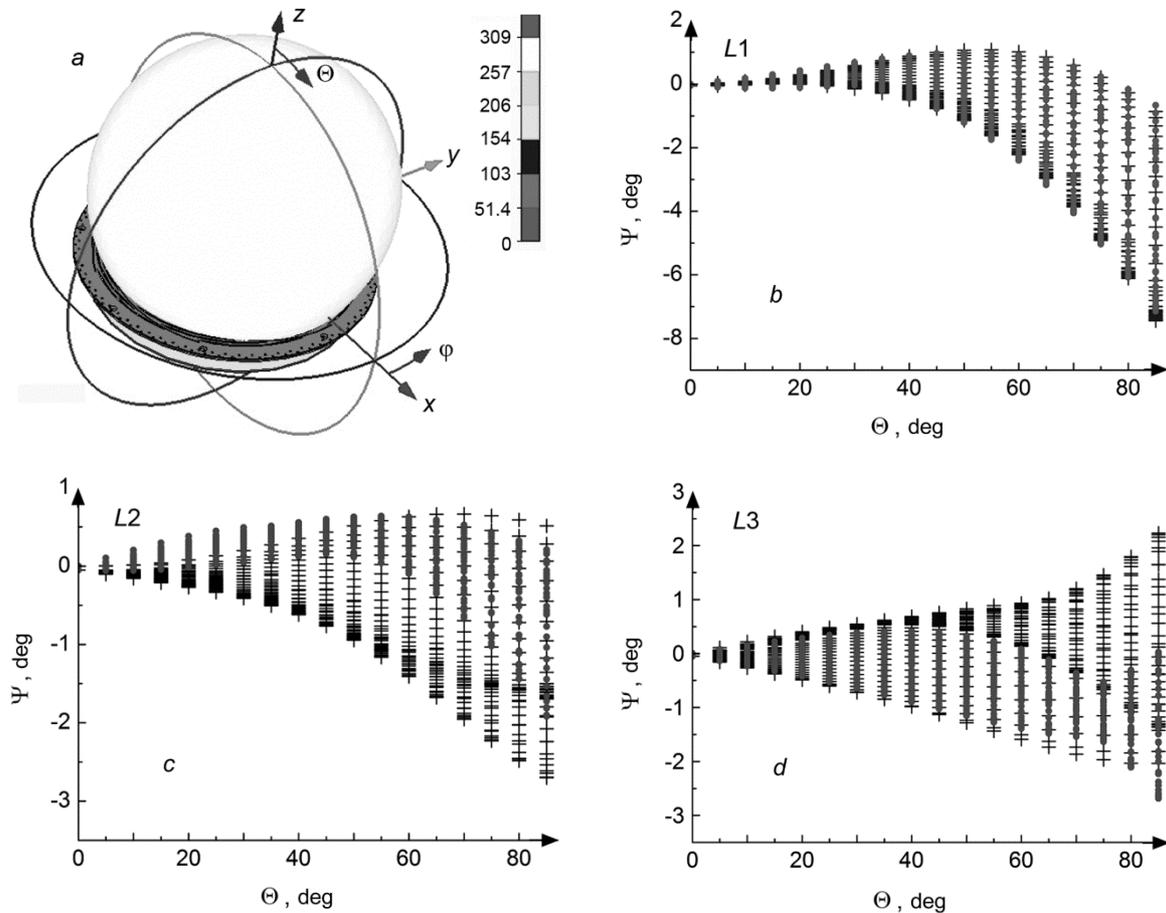
Fig. 6. Phase patterns of the antennas.
