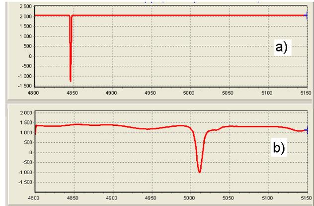
Fig. 3. Frequency dependencies of the microwave power reflected from the microwave microstrip sensor, loaded with the silicon samples with the resistivity of (a) – 2500 Ohm\*cm, and (b) – 0.06 Ohm\*cm.
